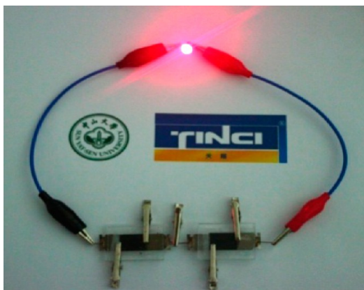
Figure 6. Red light-emitting diode (LED) lighting demonstration, with the diode driven by a simple fabricated supercapacitor.
